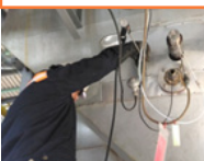
Flue Gas Temperature and Compositions Measurement
